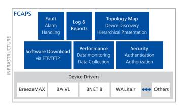
The infrastructure layer provides common functionality, including inventory, faults, topology, software download, and performance data collection. The various device drivers enable configuration and service provisioning of the particular product line being managed.
