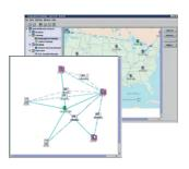
levels from regional network views down to the network element (NE). Logical topology shows visual representation of the links, interdependencies, and relationships among network devices. The physical topology provides visual representation of the actual device and any components residing inside. In addition, equipment locations can be managed according to region, cell or sector.
